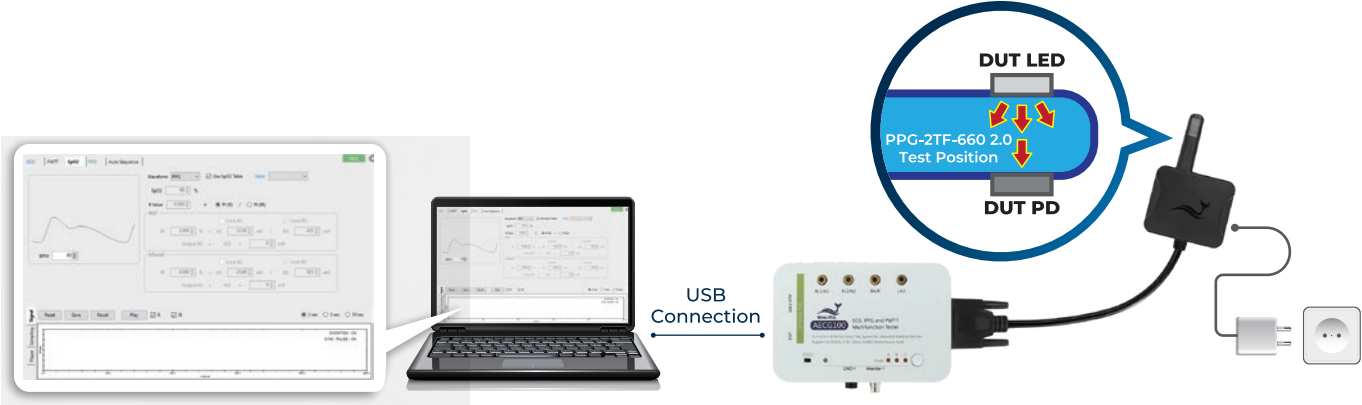
(The image illustrates the testing scenario of the PPG-2TF-660 2.0 and AECG100. Please refer to the user manual for detailed installation and instructions when using PPG-2TF-660 2.0 with AECG100 or SECG 5.0 AIO.)
